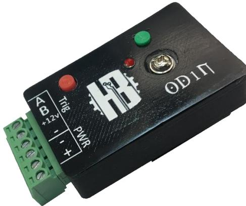
**Installation:** Remove the existing DIN connector from your solenoid valve and replace with the OD1N. The OD1N will work with any 12 to 24 Volt DC air valve.
